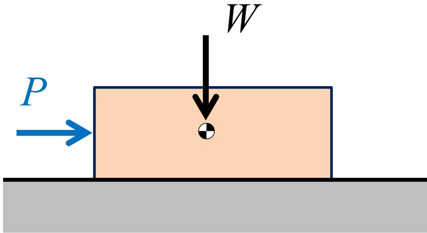
Consider a block of weight,  $W$ , sitting on a rough surface. a force,  $P$ , parallel to the surface, acts on the block.
